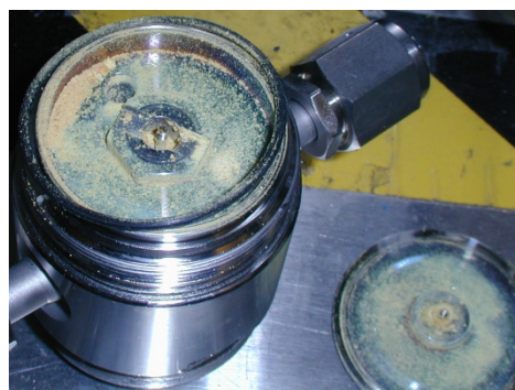
Figure 1: Picture of the first stage of diborane mixture regulator fouled with solid decomposition products.
