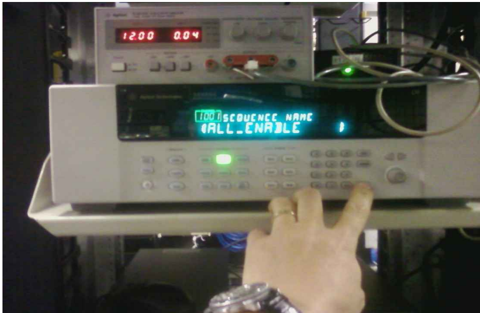
Figure 2 Going to Local mode and executing a sequence.
