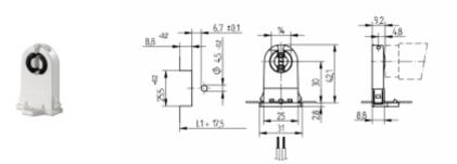
L1+17.5: Recommended cutout spacing . "L1" distance is determined by the length of the respective lamp.
