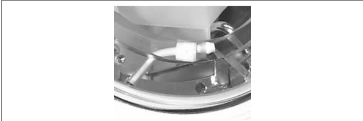
Figure 4-18. Bladder Stem with Ferrules.
