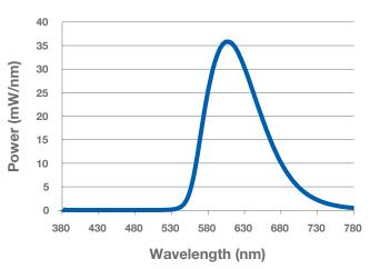
The T8 17.5W 4FT. GOLD BYP provides protection against UV rays by filtering out all wavelengths below 520nm. This lamp is an ideal choice for clean room and UV sensitive applications.
