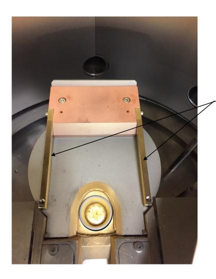
Magnets for beam optimizer
